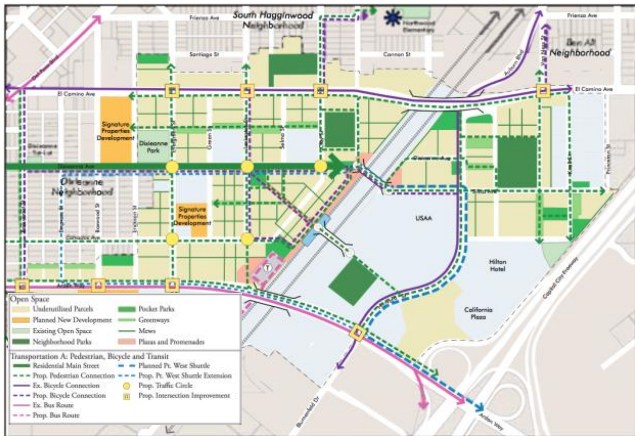
Figure 36. Proposed bicycle and pedestrian connections around Swanston station (source: City of Sacramento)
