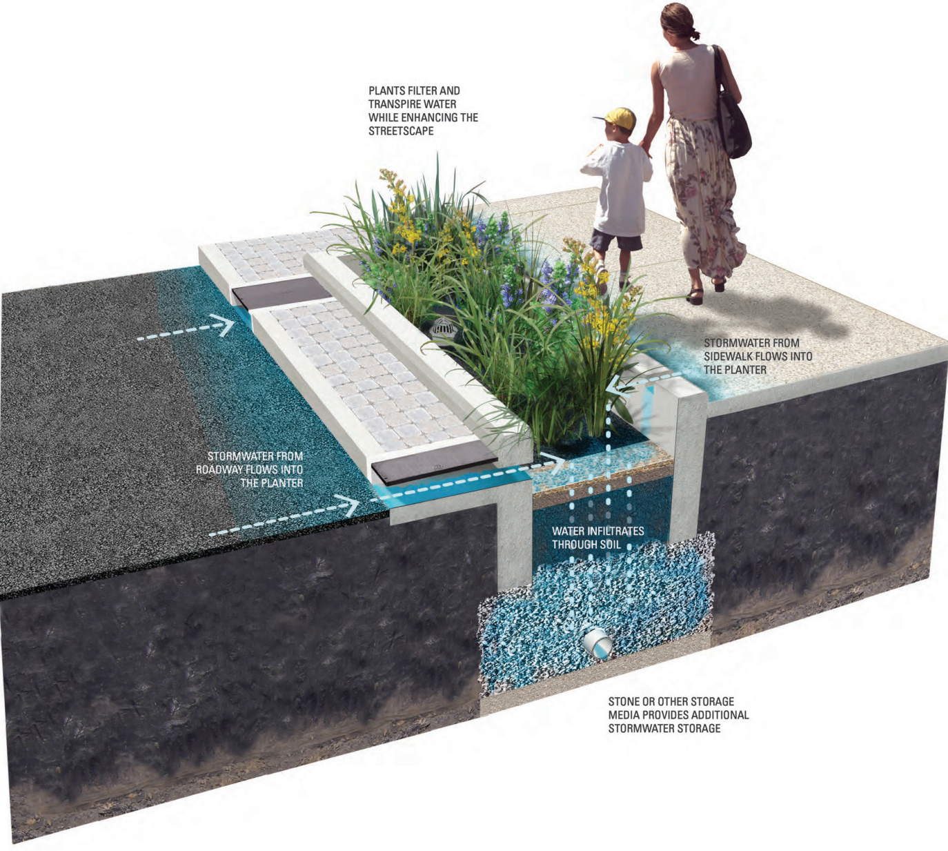
Figure 2.1: Three-Dimensional View of a Stormwater Planter
