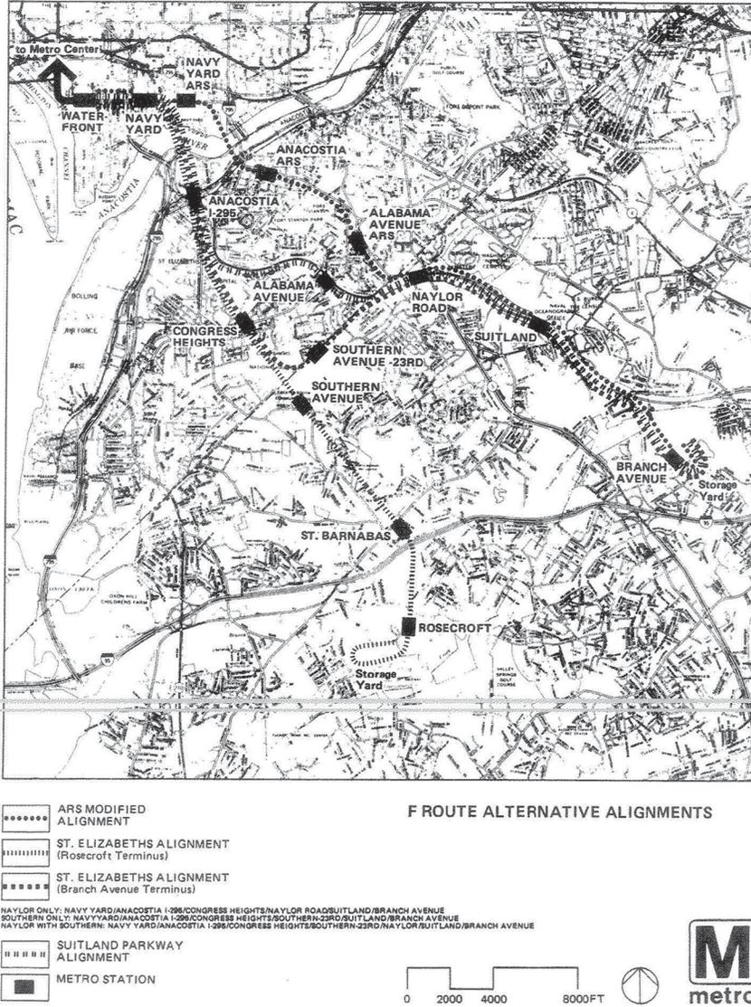
**Figure I-9: Alternative Alignments (Easternmost Infeasible Because of Navy Yard Station Location) (WMATA 1984)**
