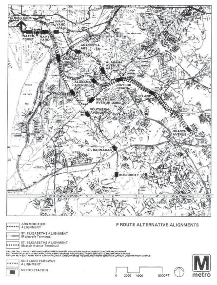
Figure I-9: Alternative Alignments (Easternmost Infeasible Because of Navy Yard Station Location) (WMATA 1984)
