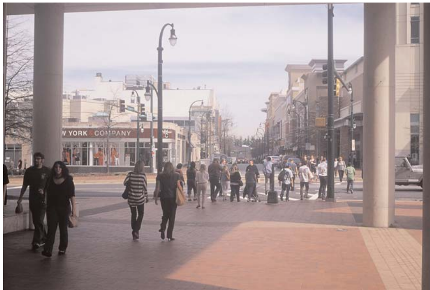
A state highway semi-mid-block (“T” intersection) signalized pedestrian crossing in combination with a pedestrian passageway provide town center access in Silver Spring, Maryland
