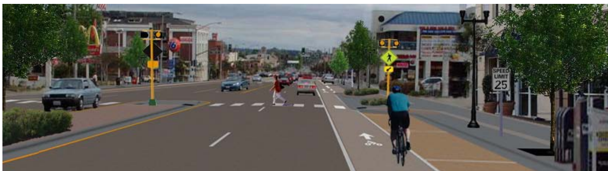
A redesigned "complete street" alternative reallocates the existing street space to better accommodate mobility and safety for all users through narrowed travel lanes; enhanced streetscape and traffic calming treatments; a lowered speed limit of 25 MPH; intermittent left-turn lanes; intermittent raised and landscaped medians with pedestrian refuge points; clearly-marked and visible pedestrian crosswalks with curb bump-outs and pedestrian-actuated signals; dedicated and clearly-delineated bicycle lanes; and relocation of sidewalk clutter to improve pedestrian travel ways and sight lines while accommodating appropriate locations and spacing for additional pedestrian-level lighting and street trees, to fit this urban context.
