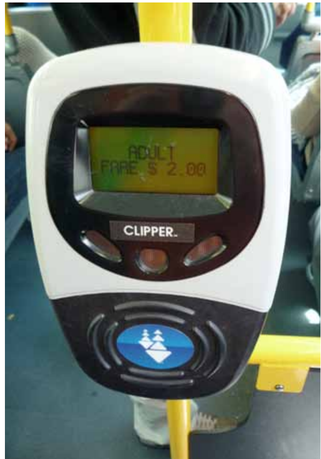
FIGURE 41 Rear-door stanchion-mounted verification device on SFMTA bus for tagging Clipper Cards.
