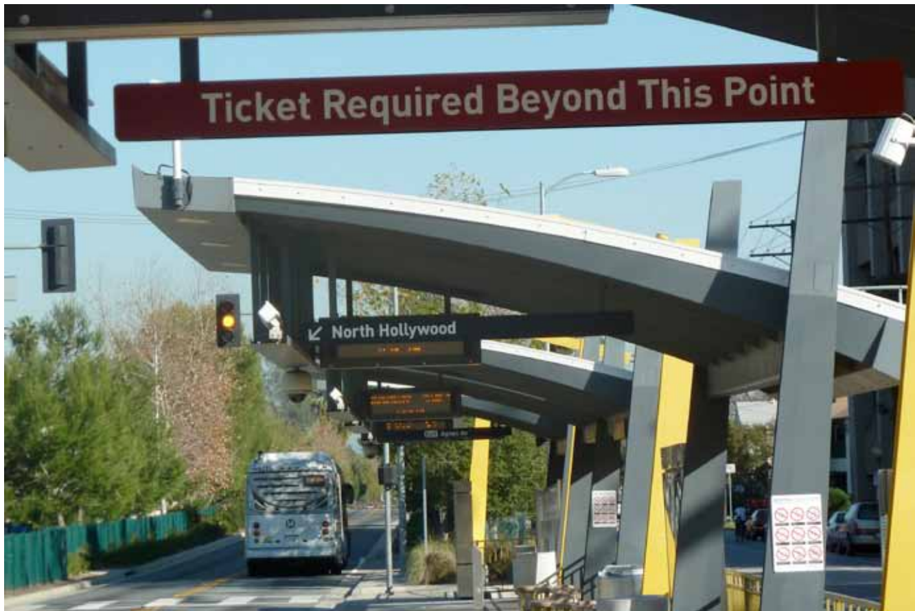
FIGURE 19 LA Metro overhead public information sign alerting passengers to PoP on Orange Line BRT platform.
