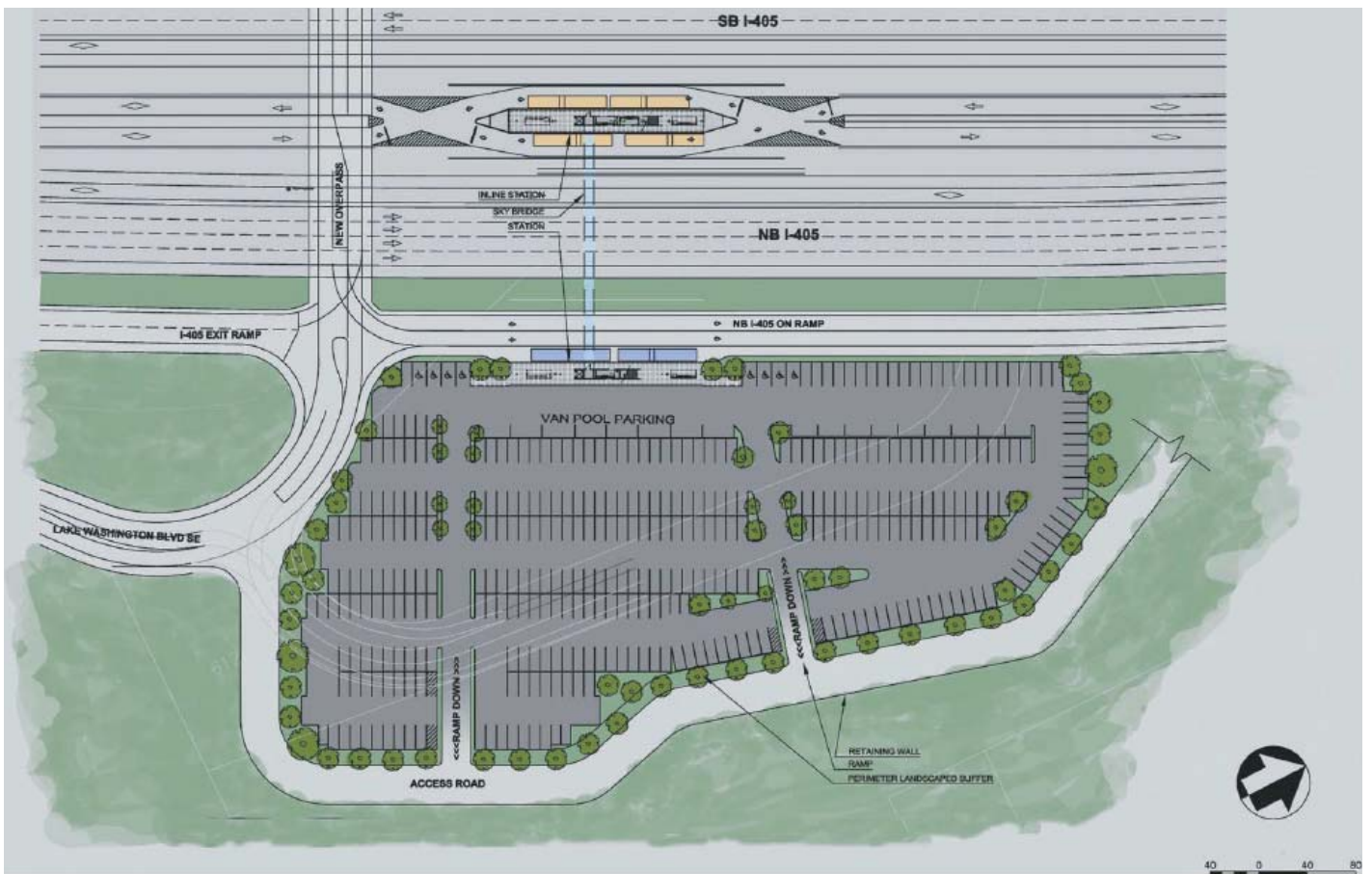
Figure 5-4. Conceptual in-median station and park-and-ride—plan view.
