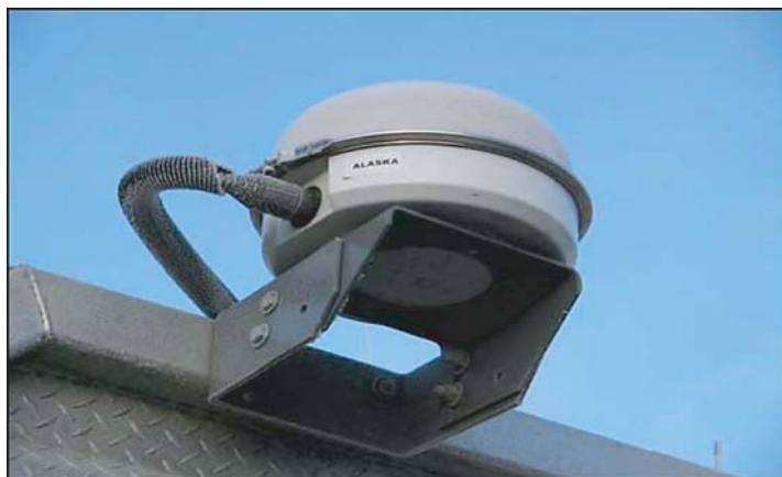
Figure 26. In-vehicle communication unit and antenna for satellite-based systems.
